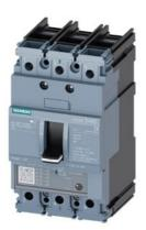
circuit breaker 3VA5 UL frame 125 3-pole, starter protection TM120M, AM, In=7A without overload protection short-circuit protection Ii=5...12 x In cable connection on both sides
