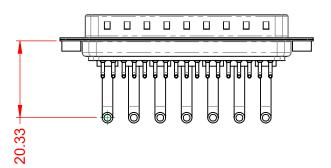
POWER/CO-AX CONTACT RATING:20A (CURRENT)(IF PRESENT)SIGNAL CONTACT CURRENT RATING:5A PER CONTACTSIGNAL CONTACT RESISTANCE: $10m\Omega$  MAX.INSULATOR RESISTANCE:5000MΩ min.DIELECTRICDIELECTRIC
