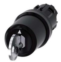
Key-operated switch IKON, 22 mm, round, plastic, lock number 360012K1, with 2 keys, 3 switch positions I>O<II, momentary contact type, actuating angle 2x45°, 10:30h/12h/13:30h, key removal O, with laser labeling, lower case
