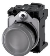
Indicator lights, 22 mm, round, plastic, clear, lens, smooth, with holder, LED module, with integrated LED 24 V AC/DC, spring-type terminal, with laser labeling, upper case
