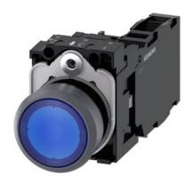
Illuminated pushbutton, 22 mm, round, plastic with metal front ring, blue, pushbutton, flat, momentary contact type, with holder, 1 NO+1 NC, LED module with integrated LED 230 V AC, screw terminal, Z=20-unit packaging
