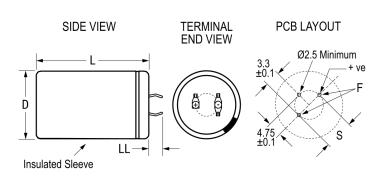
General Information Series ALC70 Dielectric Aluminum Electrolytic Description Snap-In, Aluminum Electrolytic RoHS Lead 3 Pin Short AEC-Q200 No Halogen Free Yes Component Weight 80 g Notes Dimensions D And L Include Sleeving. Shelf Life 156 Weeks
