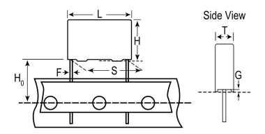
Series F461 Dielectric Metallized Polypropylene Style Radial MKP, Pulse Features RoHS Yes Lead Wire Leads AEC-Q200 No Component 2.121 g Weight The Rated Voltage Decreases 2%/C Between +85C And +105C (1.25%/C For AC). ClimCat: Miscellaneous 55/105/56. Notes Series Replaced by R75.
