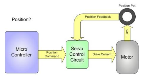
The Feedback Servos allow you to close this outer loop by providing the feedback signal to the microcontroller too!
