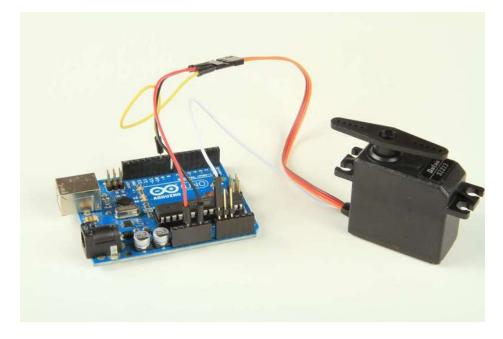
Another neat feature of feedback servos is that they can be used as an input device too! The Servo Record/Play Demo lets you record a series of servo movements, then it will replay them back for you! The recorded positions are saved in EEPROM, so they will be remembered even after resetting or powering down the Arduino
