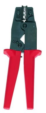
Crimping tool for non-insulated crimp lugs in flat spade shape. Easy to use, Auto-lock for proper and complete crimping, Wire can be fed in from the side, Self-opening with built-in spring.
