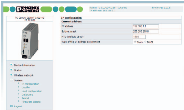
Figure 17 System, IP configuration
