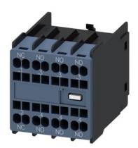
Auxiliary switch on the front, 3 NO + 1 NC Current path 1 NC, 1 NO, 1 NO, 1 NO for 3RH and 3RT spring-type terminal .1/.2, .3/.4, .3/.4, .3/.4
