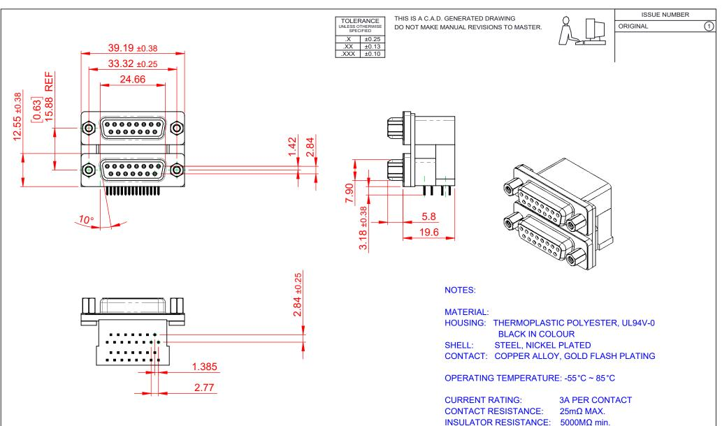
DIELECTRIC WITHSTANDING VOLTAGE: 1000V AC rms
