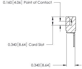
ACAD REFERENCE NO. 746 Series Ultra-Mate Card Edge Connector - Press Fit DRAWN: J.LEE Part Number: 746-022-545-501 CHECKED: **EDAC INC** SCALE: THESE DRAWINGS AND SPECIFICATIONS ARE THE PROPERTY OF EDAC INC.,AND TORONTO, ONTARIO SHALL NOT BE REPRODUCED, OR COPIED DRAWING NUMBER CANADA OR USED AS THE BASIS FOR THE 746-ENG MASTER MANUFACTURE OR SALE OF APPARATUS YOUR CONNECTION TO QUALITY & SERVICE WITHOUT WRITTEN PERMISSION.
