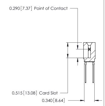
746 Series Ultra-Mate Card Edge Connector - Press Fit Part Number: 746-052-553-201
