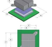
1) Dimension A is the length of the heat sink in the direction of the flow.
