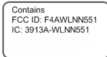
Figure 9 - Minimum FCC/IC Label
