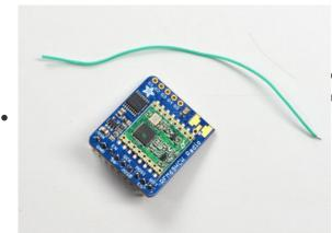
Cut a stranded or solid core wire the the proper length for the module/frequency
