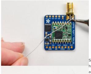
Solder in the two side ground pads. Note you will need a lot of heat for this, because the connector is an excellent heat sink and its got a huge ground plane
