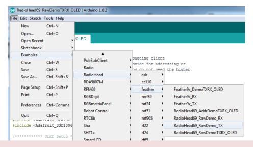
☐ Before uploading, check for the #define FREQUENCY RF69\_915MHZ line and comment that out (and uncomment the line above) to match the frequency of the hardware you're using
