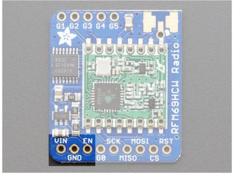
The left-most pins are used for power
