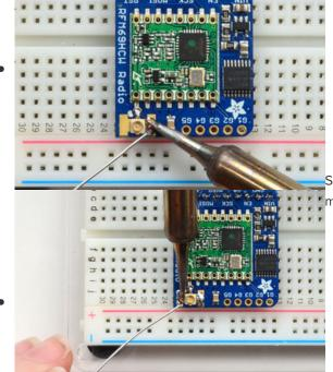
Solder in the two side pads, they are used for signal and mechanical connectivity so make sure there's plenty of solder
