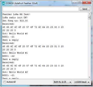
You can see that the library example prints out the hex-bytes received 48 65 6C 6C 6F 20 57 6F 72 6C 64 20 23 30 0 20 20 20 0 0, as well as the ASCII 'string' Hello World . Then it will send a reply.
