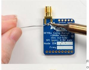
Flip over and also do the other side ground/mechanical contacts
