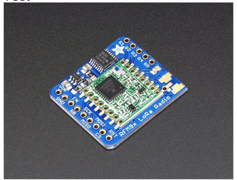
Note that the sub-GHz radio is not designed for streaming audio or video! It's best used for small packets of data. The data rate is adjustbale but its common to stick to around 19.2 Kbps (thats bits per second). Lower data rates will be more successful in their transmissions
