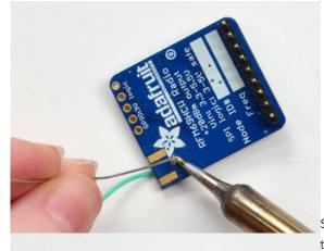
Strip a mm or two off the end of the wire, tin and solder into the **ANT** pad.
