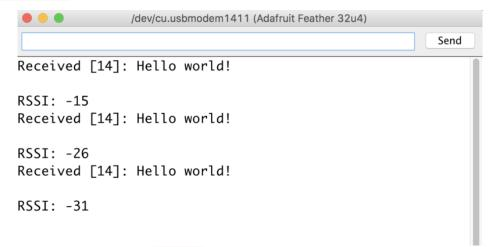
To receive a message simply call the receive function. This function will wait for half a second for any packet to be received. If a packet is found it will be returned as a byte string (remember packets are at most 60 bytes long), or if no packet was found a result of None is returned.
