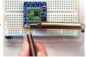
Solder in the first pad while holding the uFL steady
