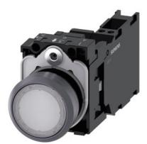
Illuminated pushbutton, 22 mm, round, plastic with metal front ring, white, pushbutton, flat, momentary contact type, with holder, 1 NO+1 NC, LED module with integrated LED 24 V AC/DC, Spring-type terminal
