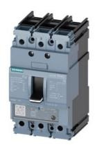
circuit breaker 3VA5 UL frame 125 breaking capacity class H 65kA @ 480 V 3-pole, line protection TM230, FTAM, In=35A overload protection Ir=35A fixed short-circuit protection Ii=5...10 x In cable connection on both sides
