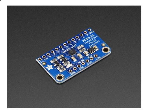
Add lots of touch sensors to your next microcontroller project with this easy-to-use 12-channel capacitive touch sensor breakout board, starring the MPR121. This chip can handle up to 12 individual touch pads.
