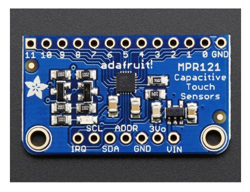
The little chip in the middle of the PCB is the actual MPR121 sensor that does all the capacitive sensing and filtering. We add all the extra components you need to get started, and 'break out' all the other pins you may want to connect to onto the PCB. For more details you can check out the schematics in the Downloads page.
