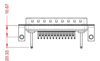
**OPERATING TEMPERATURE:** -55°C ~ 125°C 10A (CURRENT) POWER/CO-AX CONTACT RATING: (IF PRESENT) SIGNAL CONTACT CURRENT RATING: 5A PER CONTACT SIGNAL CONTACT RESISTANCE:  $10m\Omega$  MAX. **INSULATOR RESISTANCE:** 5000MΩ min.
