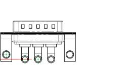
40A (CURRENT) POWER/CO-AX CONTACT RATING: (IF PRESENT) SIGNAL CONTACT CURRENT RATING: 5A PER CONTACT SIGNAL CONTACT RESISTANCE:  $10m\Omega$  MAX.
