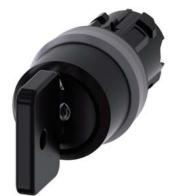
Key-operated switch O.M.R, 22 mm, round, plastic with metal front ring, lock number 73034, black, with 2 keys, 3 switch positions I>O<II, momentary contact type, actuating angle 2x45°, 10:30h/12h/13:30h, key removal O, with laser labeling, upper case
