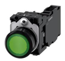
Illuminated pushbutton, 22 mm, round, plastic, green, pushbutton, flat, momentary contact type, with holder, 1 NO+1 NC, LED module with integrated LED 24 V AC/DC, screw terminal, with laser labeling, upper case
