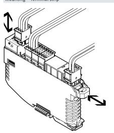
The terminal strips mounted on a module are held in position by a central locking mechanism.
