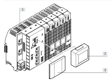
The operator unit CDSB-A1 from Festo is a plug-in display and operating panel for the automation system CPX-E. The integrated colour TFT display with touchscreen can be used both for operation and for simple diagnostics of the connected basic unit. User-friendliness is enhanced through fault diagnostics with plain-text error messages.
