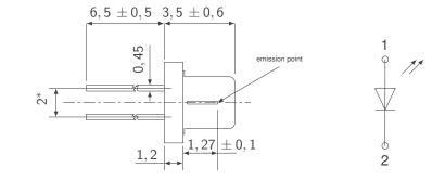
all dimensions in mm. Tolerance  $\pm 0,\,2$  except given ones \* at the bottom of the LED
