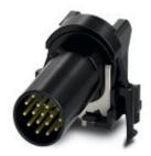
Sensor/actuator flush-type plug, 17-pos. with shroud, A-coded, with angled solder connection, contact insert only
