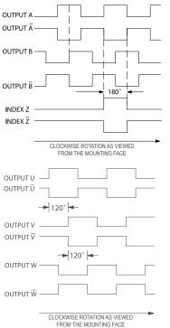
FROM THE MOUNTING FACE NOTE: ALL DEGREE REFERENCES ARE ELECTRICAL DEGREES WAVE-FORM SHOWN WITH OPTIONAL COMPLEMENTARY SIGNALS Ä, B, Ž FOR HV AND OD OUTPUTS ONLY.
