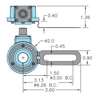
All dimensions are in inches with a tolerance of  $\pm 0.005$ " or  $\pm 0.01$ " unless otherwise specified.
