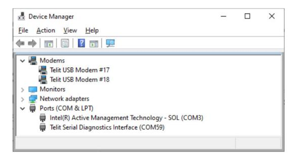
USB Modem ports are ACM devices and can be used as AT Command interface. To identify the corresponding COM port number, just right click on one of the two **Telit USB Modem** entries, select **Properties**, then **Modem** tab.
