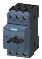
Circuit breaker size S00 for starter combination Rated current 12.5 A N-release 163 A screw terminal Standard switching capacity
