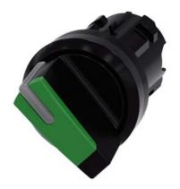
Selector switch, illuminable, 22 mm, round, plastic, green, selector switch, short, 2 switch positions O<I, momentary contact type, Actuating angle 45°, 10:30h/12h Z=50-unit packaging
