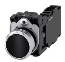
Pushbutton, 22 mm, round, metal, shiny, black, pushbutton, flat, momentary contact type, 1 NO+1 NC, screw terminal, with laser labeling, upper case and lower case, always upper case at the beginning of the word
