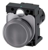
Indicator light with LED lamp, compact, 22 mm, round, plastic, clear with red-yellow-green LED, lens, smooth, with holder, operating voltage 6-24 V AC/DC, screw terminal, with laser labeling, upper case
