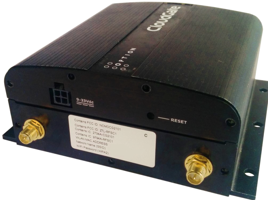
Figure 2: Monnit expansion card with Wi-Fi (CG2104) installed on CloudGate.
