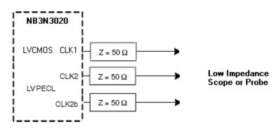
Figure 7. Typical Device Termination Setup and Termination for Split Supply Operation (50  $\Omega$  Low Impedance Scope or Probes)
