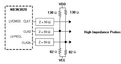
Figure 8. Alternative Device Termination Setup for On-Board Termination
