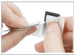
Remove the push-button label from the carrier film. Press and hold the pre-punched carrier film to do this.
