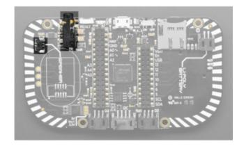
There is a speaker connector on the left side of the back, which is a Molex PicoBlade (). You can attach one of the speakers available in the Adafruit shop. There is also a stereo headphone jack on the left top.
