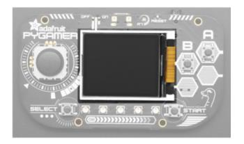
1.8" TFT display - The front features a 160x128 pixel color display.
