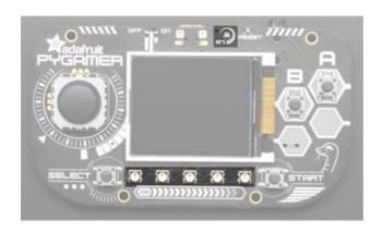
Light sensor (A7) - There is an ambient light sensor on the top, which points through to the front. The light sensor is an analog input, connected to board.LIGHT (CircuitPython) or A7 (Arduino) you can read it as any analog value ranging from 0 (dark) to 1023 (in Arduino) or 65535 (CircuitPython) when bright.
