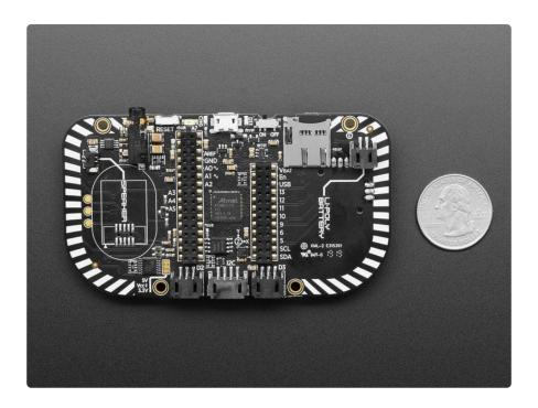
For built in sensors, there's a light sensor that points out the front, and a 3-axis accelerometer that can detect taps and free-fall. To make bleeps and bloops, plug in any set of stereo headphones. For projects where you need more volume, you can plug in one of our 8 ohm speakers (). The PyGamer will auto-switch to speakers when they're plugged in.
