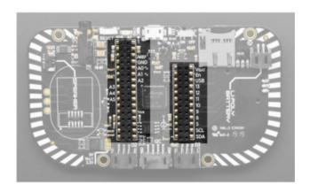
You can easily attach FeatherWings to the back of your PyGamer using the convenient "Feather Headers" on the back. Located in the middle, they break out all the same pins you have access to on a Feather board, allowing use of any of our wide range of FeatherWings. Easily add all kinds of functionality to your PyGamer! The GPIO is all 3.3V logic.
