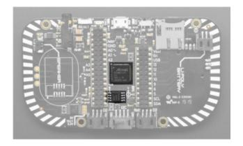
The main processor chip is the ATSAMD51J19 Cortex M4 running at 120MHz with 3.3v logic/power. It has 512KB of Flash and 192KB of RAM. We also include 8 MB of QSPI Flash for storing images, sounds, animations, whatever.
