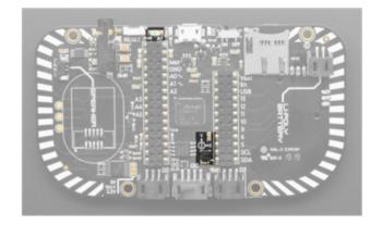
Accelerometer - There is an accelerometer located near the middle, above the I2C connector. It is an LIS3DH.
