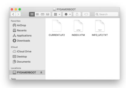
The bootloader version is listed in <a href="INFO\_UF2.TXT">INFO\_UF2.TXT</a>. In this example, the version is v3.6 .0.
