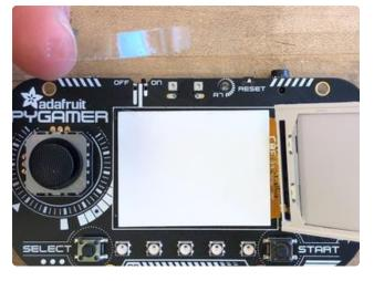
The small bits of adhesive may have given up the fight. Go ahead and lift the screen away from the backing, being careful to go gentle on the ribbon connector!
