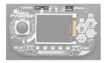
On/Off switch - Powers off the board. Even if plugged in, the board won't work if switched to off. You can charge the battery when the board is off, but the USB device will not be active or any other electronics. The reset button is located on the top to the right of center. Click it once to re-start your firmware. Click twice to enter bootloader mode.
