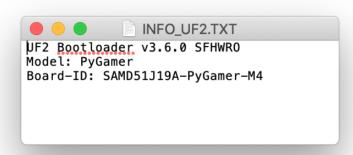
If the bootloader version you see is smaller than "v3.9.0", you need to update. For instance, the bootloader above needs to be upgraded.
