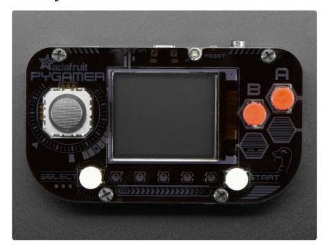
Here's how to assemble the laser cut acrylic case for the PyGamer. The kit comes with seven pieces of acrylic, and four screws and nuts. You've got ten button caps to pick from (you'll pick four), and you'll also want to connect the speaker and battery for the full portable experience.
