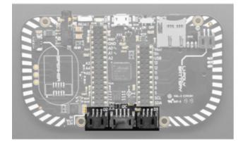
There is a 4-pin JST PH 2.0mm I2C connector in the center on the bottom, that is STEMMA and Grove compatible as well as Stemma QT with an adapter cable (). You can access VCC power and ground as well as a level-shifted SDA & SCL connection. In CircuitPython, you can use the STEMMA connector with board.SCL and board.SDA, or board.STEMMA\_I2C(). You can change VCC from 5V (default) to 3V by cutting/ soldering the solder jumper to the right of the D3 connector.
