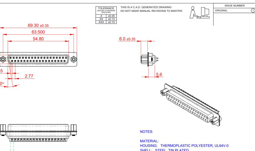
SHELL: STEEL, TIN PLATED CONTACT: COPPER ALLOY, 30µ GOLD PLATED OPERATING TEMPERATURE: -55°C to +105°C
