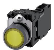
Illuminated pushbutton, 22 mm, round, plastic with metal front ring, yellow, pushbutton, flat, momentary contact type, with holder, 1 NO+1 NC, LED module with integrated LED 24 V AC/DC, screw terminal, with laser labeling, inscription or symbol Customer-specific selection with SIRIUS ACT configurator (CIN)
