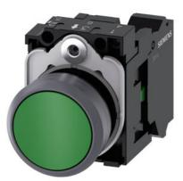
Pushbutton, 22 mm, round, plastic with metal front ring, green, pushbutton, flat, momentary contact type, with holder, 1 NO, spring-type terminal, with laser labeling, upper case
