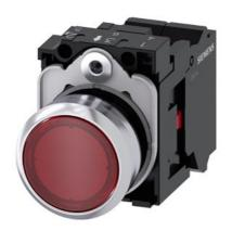
Illuminated pushbutton, 22 mm, round, metal, shiny, red, pushbutton, flat, momentary contact type, with holder, 1NC, LED module with integrated LED 110 V AC, spring-type terminal, with laser labeling, upper case and lower case, Always upper case at the beginning of the word
