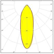
Dimensions: 18.0 mm x 18.0 mm Height: 5.00 mm ~35° spot beam
