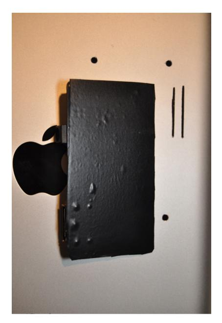
Okay, you're ready to attach the Qualia! Put a 2x8mm screw through each of the holes for the Qualia in the back panel, with the heads on the *inside* of the iPad. Place a #2 plastic washer on each of the machine screws. Now, drop the Qualia board onto the screws, and secure it with the #2 metric hex nuts.
