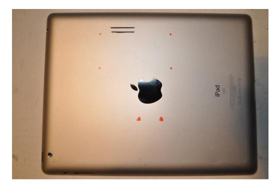
If you're happy with how the marks look, go ahead and drill 'em! The two large holes are #3 Metric, and the smaller ones are for the #2. Be careful not to overdrill the holes.
