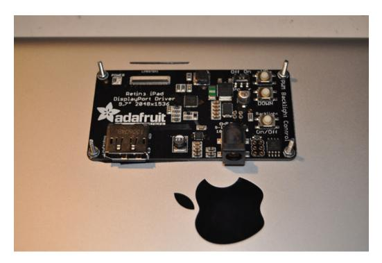
Place a #3 washer on each 3x12mm machine screw. Then, thread those through the iPad back panel, with the heads on the inside of the case (same as before). Place your back panel onto the lamp head, and thread the screws through the bracket. place your #3 crush washers onto the screws, then another set of #3 plastic washers, and finally cap them with the #3 metric hex nuts. Tighten it up, and it's mounted!
