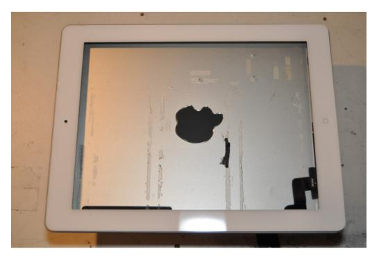
The Retina Display will clash with the Back Panel in the two corners that are on the same side as the rear facing camera. The corner that is closer to the rear facing camera will have to have some of the aluminum removed. Grab your Dremel, and cut along the orange line I have marked in this photo.
