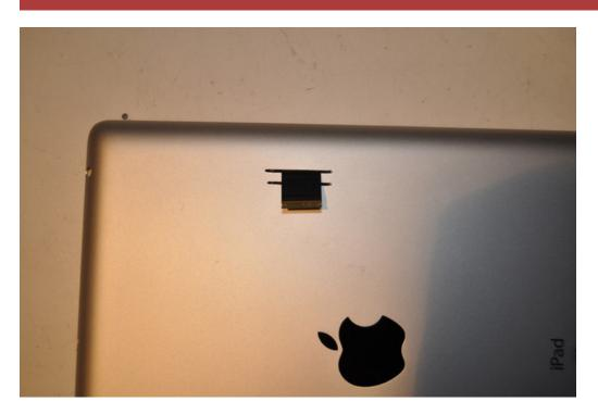
Using the ribbon as your guide, place your Qualia bareboard where you should mount it on the back of the iPad back panel. The ribbon should not flex or bend in a strange way. Try to align it so that it goes straight into the Qualia.
