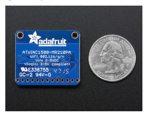
This module works with 802.11b, g, or n networks & supports WEP, WPA and WPA2 encryption. The datasheet says it can do Soft-AP mode but we don't have any code to actually use that.
