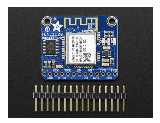
Comes with a stick of header you can solder on, to plug into a breadboard and a set of tutorials & code so you can follow along!
