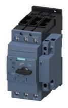
Circuit breaker size S2 for motor protection, CLASS 10 with overload relay function A-release 14...20 A N-release 260 A screw terminal Standard switching capacity
