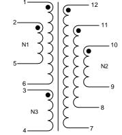
N1, N2 denotes windings connected in parallel. Terminals 1+2, 5+6, 7+8+9 and 10+11+12 must be tied as solder bridging is allowed.
