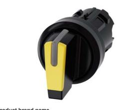
Selector switch, illuminable, 22 mm, round, plastic, yellow, selector switch, short, 3 switch positions I-O-II, latching, actuating angle 2x45°, 10:30h/12h/13:30h, with laser labeling, upper case and lower case, always upper case at the beginning of the word
