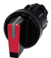
Selector switch, illuminable, 22 mm, round, plastic, red, selector switch, short, 3 switch positions I-O<II, left latching, right momentary contact type, actuating angle  $2x45^{\circ}$ , 10:30h/12h/13:30h, with laser labeling, upper case and lower case, always upper case at the beginning of the word
