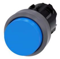
Pushbutton, 22 mm, round, plastic with metal front ring, blue, pushbutton, raised momentary contact type, with laser labeling, upper case and lower case, always upper case at beginning of line
