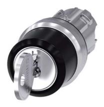
RONIS key-operated switch, 22 mm, round, metal, shiny, special lock, with 2 keys, 3 switch positions I-O<II, left latching, right momentary contact type, actuating angle  $2x45^{\circ}$ , 10:30h/12h/13:30h, key removal O+I, possible special locks: SB31, 421, 455
